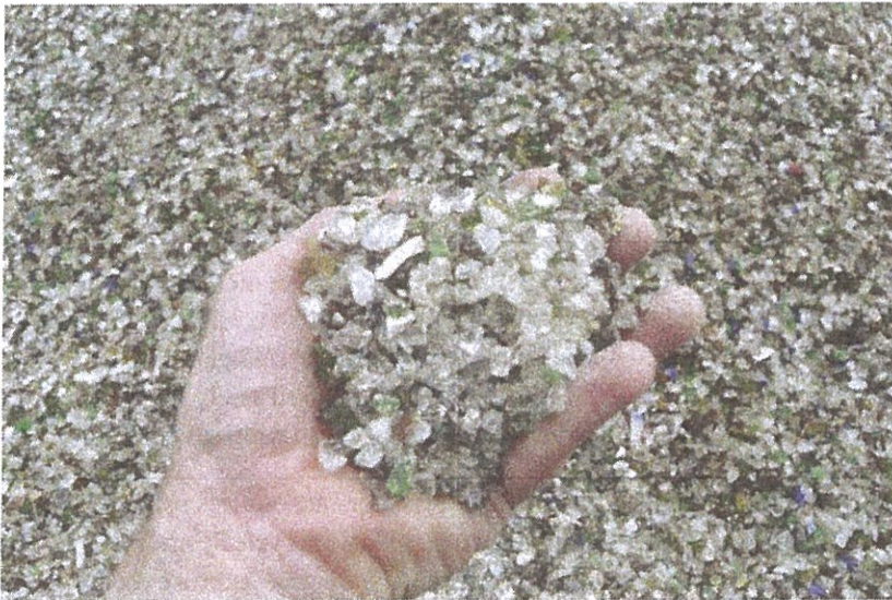
Recycled glass bottles are turned into "gravel" (shown above) and "sand" after processing with the Andela Pulverizer.
