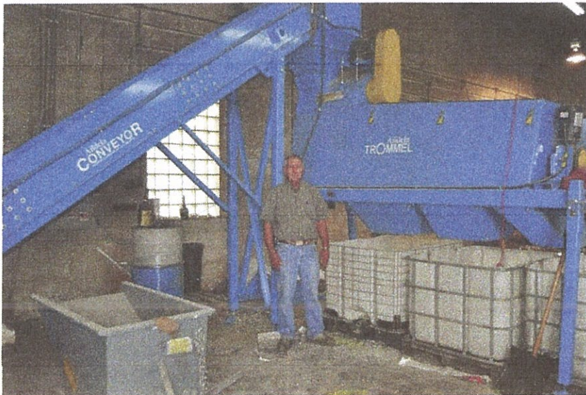
Tom Breeden, Cumberland County Solid Waste Director, demonstrates the Andela "Friendly Glass" Pulverizer machine, which he credits for more than doubling the rate of glass recycling in Cumberland County in less than one year.
